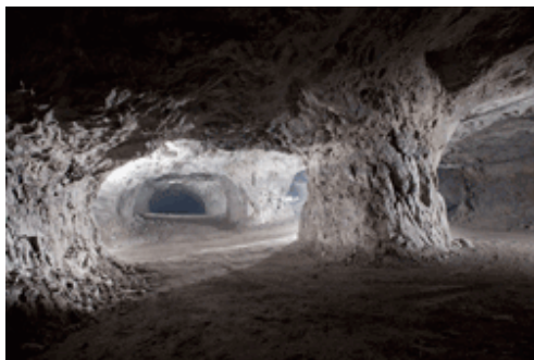
Minersa's Mina Moscona, Spain, showing chambers and pillars in a worked-out area of the stratiform mineralisation
